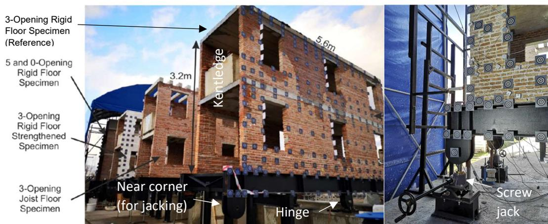
Figure 1 – The experimental setup and specimens.
