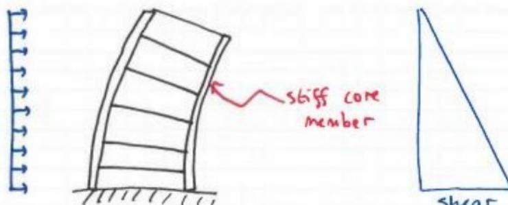
The perfectly rigid lintels (causing the 'stiff core members' to act compositely) transfer the shear between 'stiff core members'.
