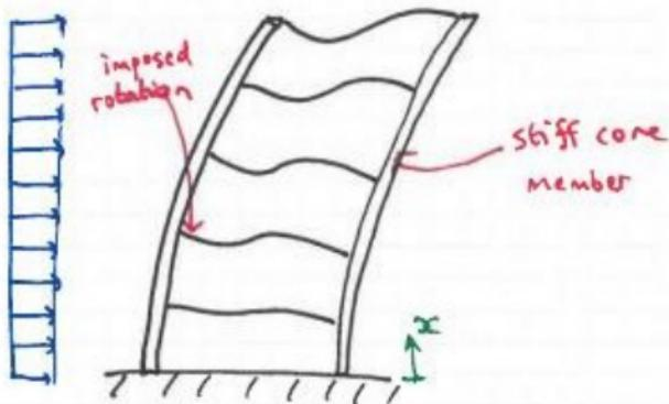
For perfectly flexible lintels, the moment in each 'stiff core member' scales:
