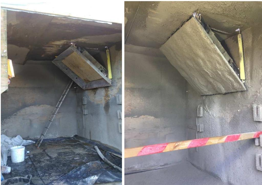
**Figure 2: Sprayed concrete panels from Ecocem and Shotcrete trials**
