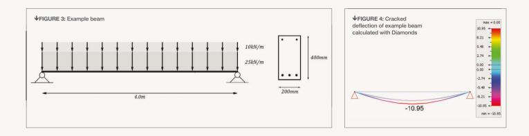
For reinforced concrete elements, the curvature value 1/r depends on whether or not the crosssection is cracked. A cross-section is cracked only when the bending moment exceeds the cracking moment  $M_{.}$  The cracking moment  $M_{.}$  is determined by
