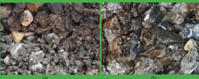
Figure 3. Uncoated and coated aggregate after sulfate soundness test
