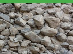
Figure 4. RCA after LA abrasion test
