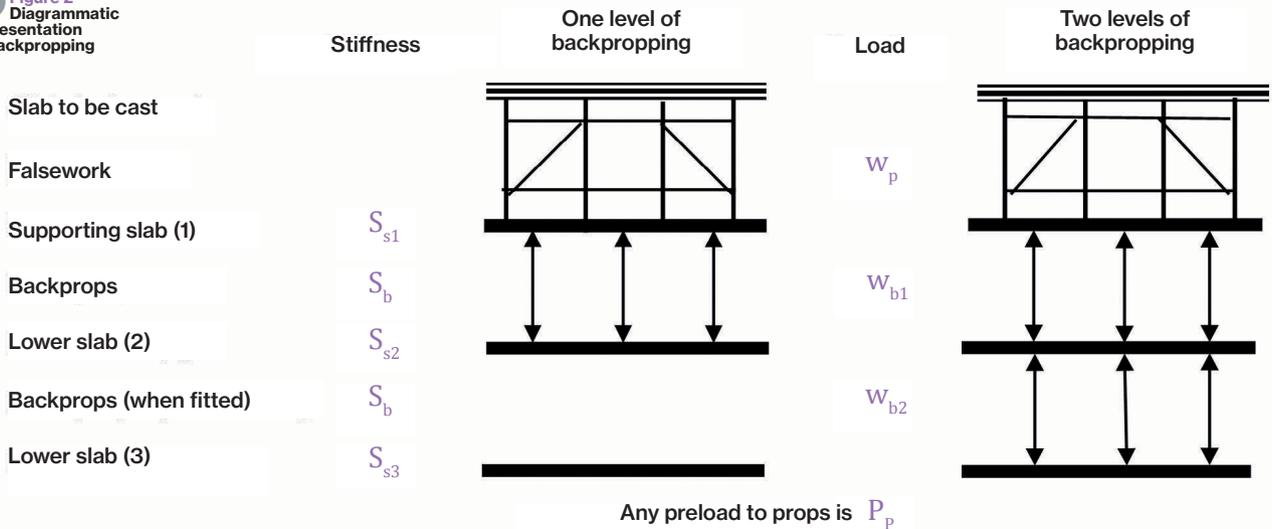
act as a distributed load, or as individual point loads from each of the falsework legs? Further, the grid of backprops below the supporting slab, transferring load to lower floors, will rarely be at the same centres as the falsework legs (only about a third of the load is transferred); hence, the concrete supporting slab will also have an influence on load transfer.
