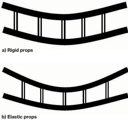
pre-tensioned props which would push the floor above upwards, decreasing its load, while at the same time increasing the load into the lower floor. The nomenclature usually used for backpropping relating to the varying stiffness is shown in Figure 2.
