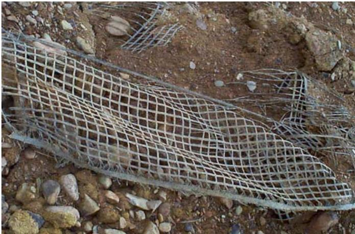
Figure 24: At some locations, the geotextile failed in tension
