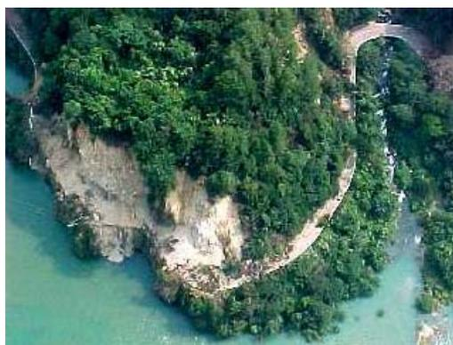
Figure 20: Blocking of hill roads due to landslides
