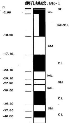
Fig.12 Soil classification based on bore hole data
