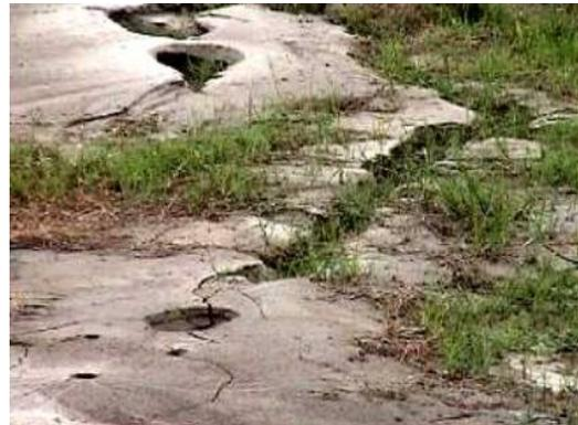
Figure 18: Sand boils at the new Nantou Hsou-Shi bridge site
