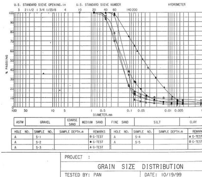
Fig.11: Particle size distribution of soil from the well in Fig.10, (courtesy A J Brennan, Research Student, Cambridge University)
