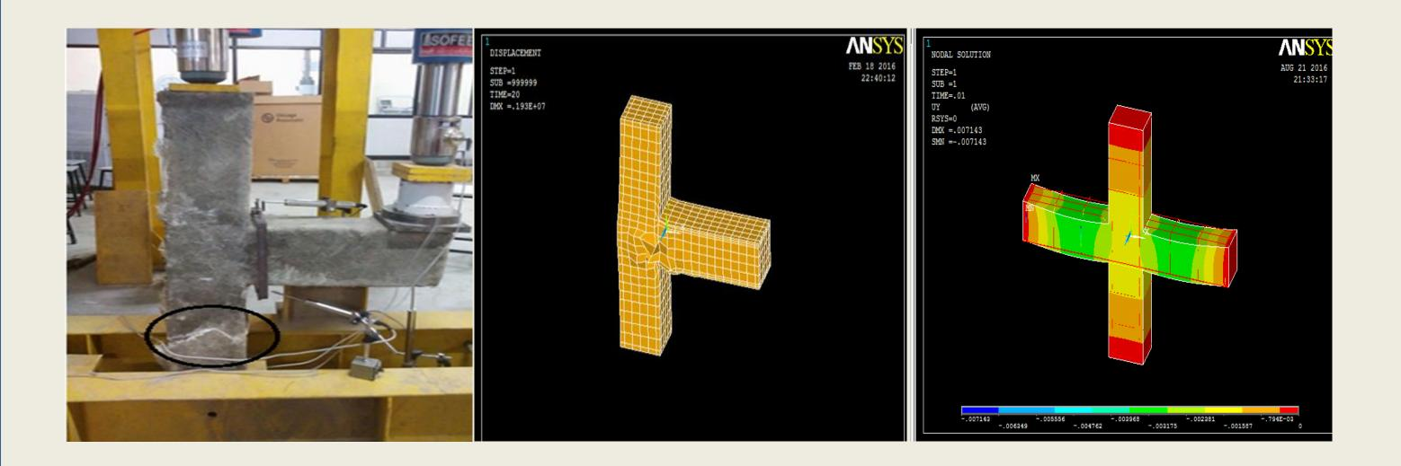
Figure 4. Crack pattern with FRP<br/>wrapping.Figure 5. Crack pattern with FRP<br/>wrapping ANSYS.
