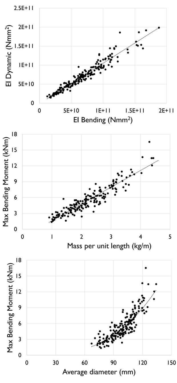
Mass per unit length and average external diameter were selected as strong indicating properties for flexural stiffness and flexural capacity and two possible grading systems are proposed; using diameter alone, and a combined method using both diameter and mass per unit length.
