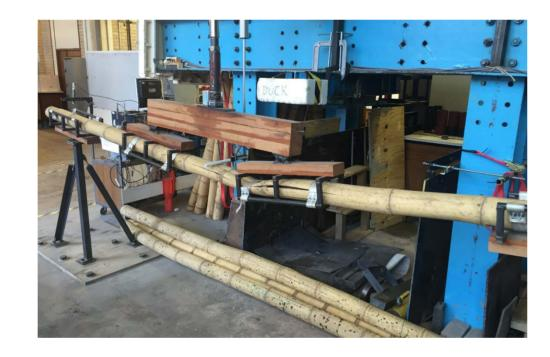
Specimens were loaded at a rate of 0.5m/s and deflection was measured at the mid-point and supports.
