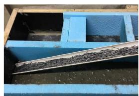
Steel fibre alignment
