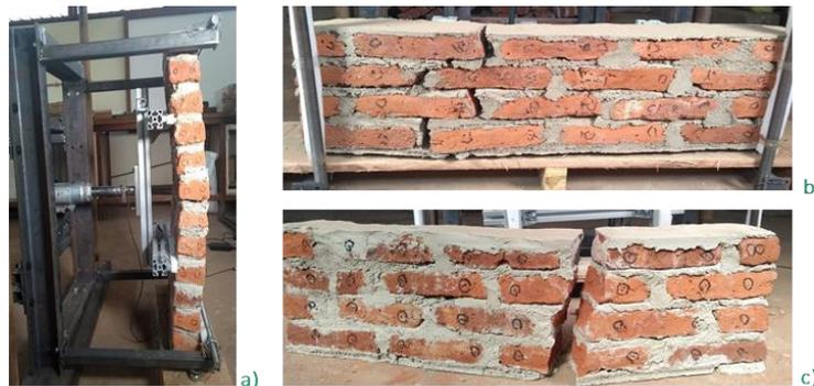
*Figure 12: Out-of-plane flexural failure modes: (a) parallel and (b) perpendicular to the brick bending.*
