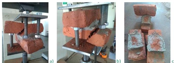
*Figure 10: Compressive tests and related failure modes for masonry prisms; note the local brick crushing mechanism in the bottom pictures.*
