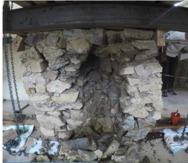
Figure 33. Delamination of the SMM wall specimen at ultimate state (Build Change, 2019).
