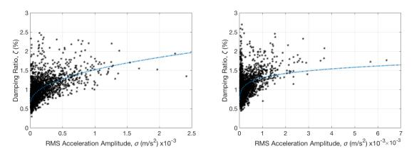
Figure 6. Relationship between damping ratio of the first mode and the corresponding RMS acceleration amplitude in the x (left hand-side plot) and y directions (right hand-side plot).
