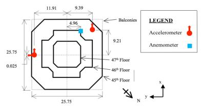
Figure 1. Plan of the top three floors of tower showing locations of instruments and local coordinate system (dimensions in m).
