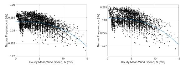
Figure 7. Relationship between first natural frequency and the corresponding 1-hour mean wind speed in the x (left hand-side plot) and y directions (right hand-side plot).
