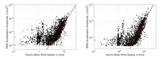
Figure 4. Relationship between modal RMS acceleration amplitude and the corresponding 1-hour mean wind speed in the x (left hand-side plot) and y directions (right hand-side plot).
