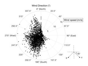
Figure 3. Polar plots of 1-hour average wind velocities.
