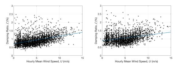
Figure 5. Relationship between damping ratio of the first mode and the corresponding 1-hour mean wind speed in the x (left hand-side plot) and y directions (right hand-side plot).
