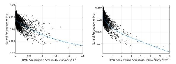
Figure 8. Relationship between first natural frequency and the corresponding RMS acceleration amplitude in the x (left hand-side plot) and y directions (right hand-side plot).
